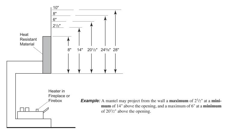
Figure 7 - Minimum Mantel Clearance with No Hood -NB18
